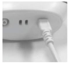
Step 8: Connect the power adaptor (15) to the pump motor (8)
