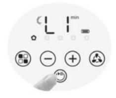
Step 9: Press the power switch by holding it in for 2 - 3 seconds
